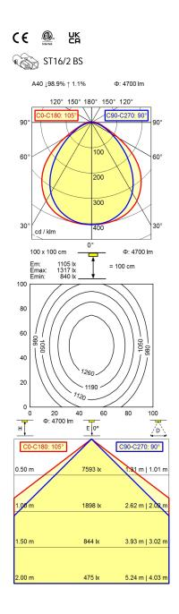
Light source LED Without Work equipment **Connected load** 22 - 26 V; DC **Power consumption** ca. 62,5 W Luminous flux approx. 4.700 lm Luminous efficiency 1) approx. 74 lm/W Light type/-color Cold white Colour temperatur approx. 5.000 K Color rendering index CRI ≥ 80 Light distribution Direct **Direct ratio** approx. 99 % Beam angle 100° **Chromaticity tolerance LED** < 4 SDCM Glare control Diffusor Luminance (L65)  $< 14.000 \text{ cd/m}^2$
